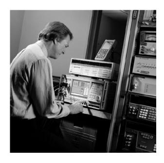
When calibrating power measurement instruments, the Fluke 6100A Electrical Power Standard has the ability to display the resultant real power (watts), apparent power (S) and reactive power (Q). These three values are often referred to as the Power Triangle.
